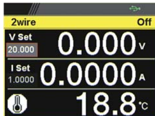
White: Temperature Control on with GTL-205A Connected
